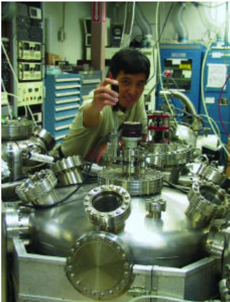
Dr. Xi Li working on the multi-chamber vacuum system used for plasma processing of materials. Various plasma devices are connected to a ultra-high vacuum sample transfer system and a multi-technique surface analysis apparatus.
