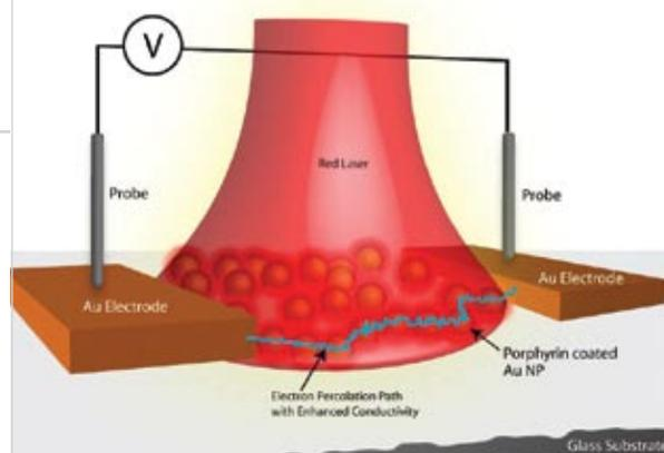
A SCHEMATIC OF A HYBRID MOLECULAR DEVICE SHOWS METAL ELECTRODES CONNECTED BY A PERCOLATION PATHWAY COMPOSED OF DITHIOL-PZn<sub>3</sub>-COATED AU NANOPARTICLES.
