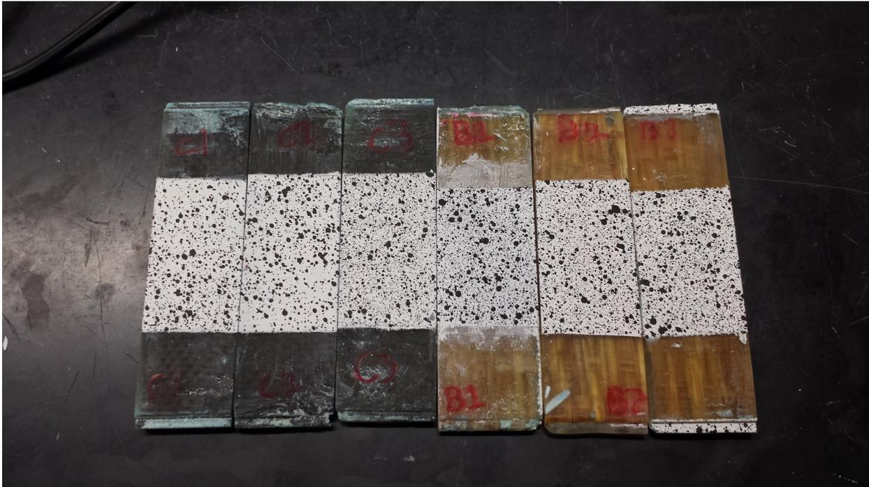
Figure 7: Samples with primer and black speckles prior to tensile test
