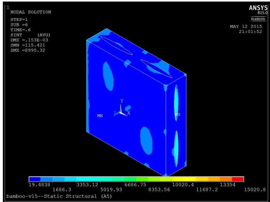
Figure 6: A snapshot of the stress intensity during a tensile test. This picture shows a point in time in the middle of the tensile test
