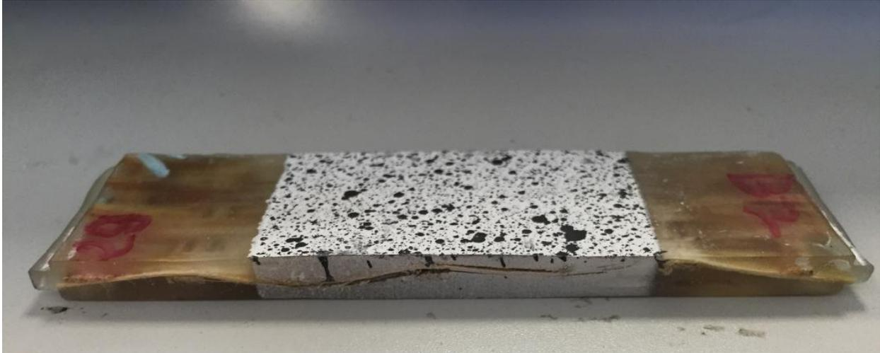
Figure 9: BFRP sample that fractured along its side due to poor fiber/epoxy adhesion
