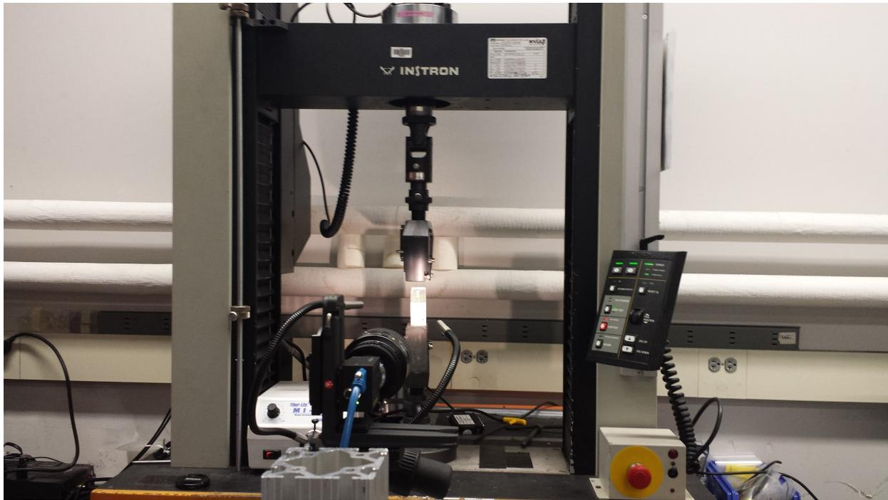
Figure 8: Experimental setup of the tensile test with camera in place
