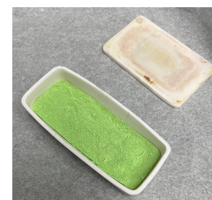
About 15g of LPNWO powder remained after calcination. The powder's color matches the bright green of the W oxide precursor.
