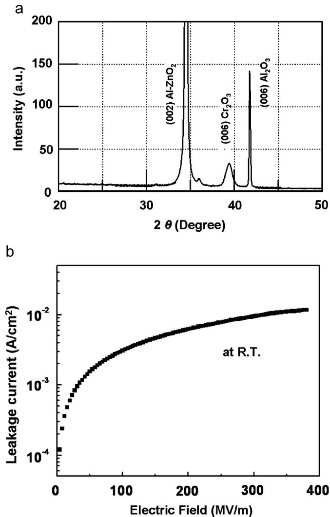
**Fig. 1.** (a) XRD  $2\text{-}\theta$  scan of a Co/Pt/Al-ZnO/Cr<sub>2</sub>O<sub>3</sub> film. (b) The leakage current density of Cr<sub>2</sub>O<sub>3</sub> film was measured using Pt (top) and Al-ZnO (bottom) electrodes at room temperature. The observed highly insulating properties of Cr<sub>2</sub>O<sub>3</sub> film were suitable for applying high electric field.
