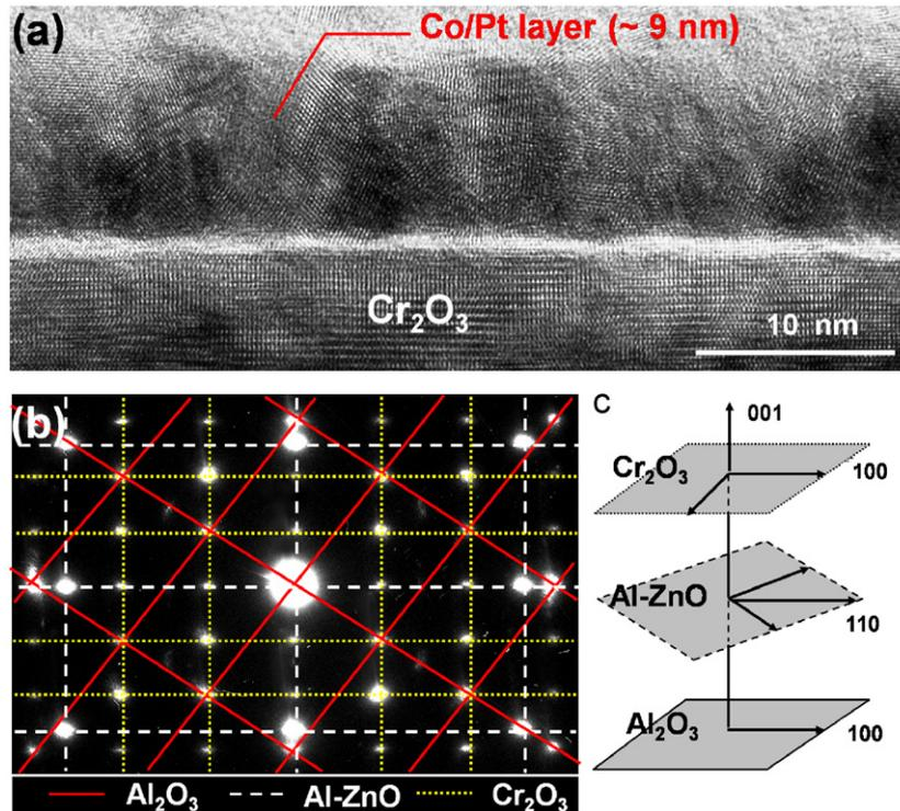
Fig. 2. (a) High-resolution TEM image of Co/Pt layer. Co particles were embedded in Pt matrix. The thickness of Co/Pt layer was ~9 nm (including the top Pt capping layer of ~2 nm). (b) The electron diffraction patterns and (c) schematics of crystal orientation relation. The film showed epitaxial growth of Al-ZnO, Cr<sub>2</sub>O<sub>3</sub> layer on c-axis sapphire substrate.
