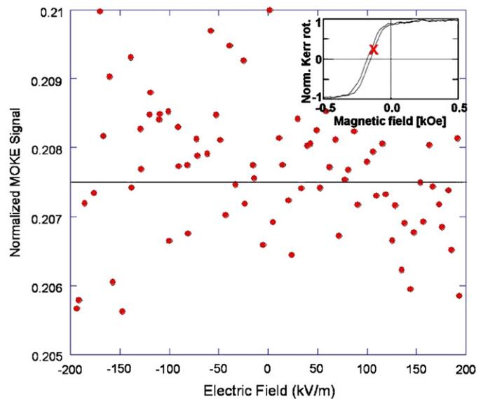
Fig. 4. Electric field versus MOKE signal measured at room temperature while the applied magnetic field is kept constant so that the system is at the “x” position in the hysteresis curve as shown in inset. The multilayer was field cooled through the Néel temperature. The vertical scale is the same as in Fig. 3(a), but magnified to display the limit of the MOKE measurement sensitivity. For this plot, the electric field was swept from 200 to -200 kV/m.
