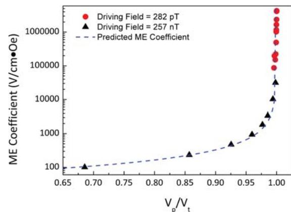
FIG. 4. Parametric amplification theory and experiment: The experimental ME coefficient (black triangles) and the theoretical ME coefficient curve (blue dashed line) as a function of pumping voltage for a driving field of 257 nT. The theory curve is plotted from Eq. (7) with  $V_t = 1.166$  V. Red circles show data at the minimum driving magnetic field (282 pT) with the current measurement setup.
