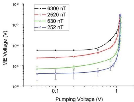
FIG. 3. The ME signals as a function of the pump voltage for different driving fields (252 nT, 630 nT, 2.52  $\mu$ T, and 6.30  $\mu$ T). Lines are not theoretical fitted lines but just guidelines. The error bars stand for the noise.
