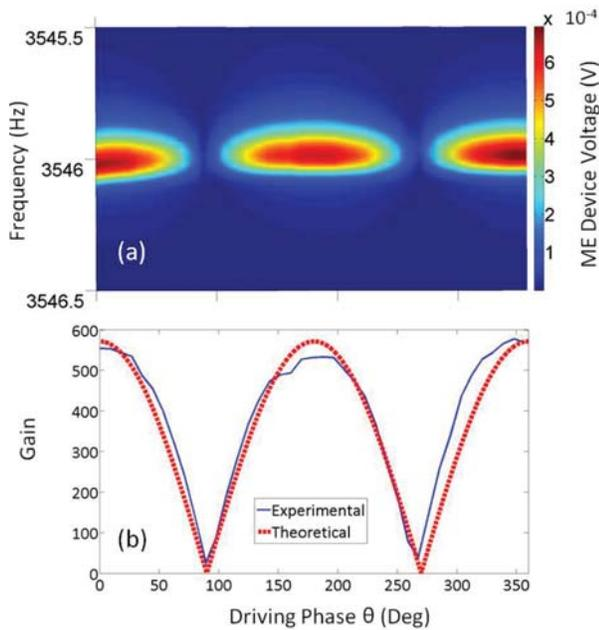
FIG. 2. ME device voltage as a function of driving parameters. (a) ME signal vs. driving phase with pumping phase set to zero. (b) Parametric gain for (a) at the resonance frequency. The driving magnetic field amplitude was approximately 257 nT, and the pumping voltage amplitude was approximately 1.16 V.
