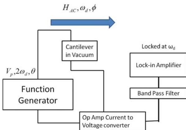
FIG. 1. Block diagram showing a multiferroic cantilever driven by a magnetic-field at angular frequency  $\omega_d$  and parametrically pumped by a voltage at  $2\omega_d$ . The response of the cantilever at angular frequency  $\omega_d$  is measured by a lock-in amplifier.
