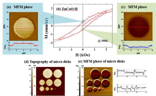
Fig. 3 MFM results (a) and (c) of a H-ZCO microdisk corresponding to certain positions along the  $M-H$  curve (b). MFM image (a) in the absence of an external magnetic field after applying an external magnetic field of +1000 Oe and (c) in the absence of an external magnetic field after applying an external magnetic field of -1000 Oe to reverse the spin-ordering along the out-of-plane direction. (d), (e) AFM and MFM results of microdisks with different sizes, respectively.
