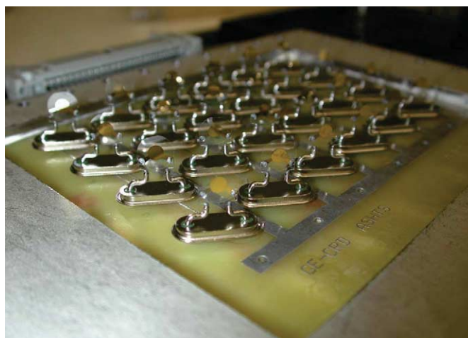
Fig. 8 A 24 channel acoustic wave sensor array for the parallel measurement of coatings performance properties. (Reprinted with permission from 112 . © 2004 Wiley-VCH.)
