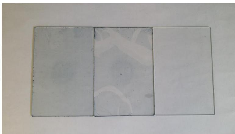
**Figure 11:** From left to right; final spin coated PEDOT:PSS film, attempt at spin coating multiple layers, and control glass slide
