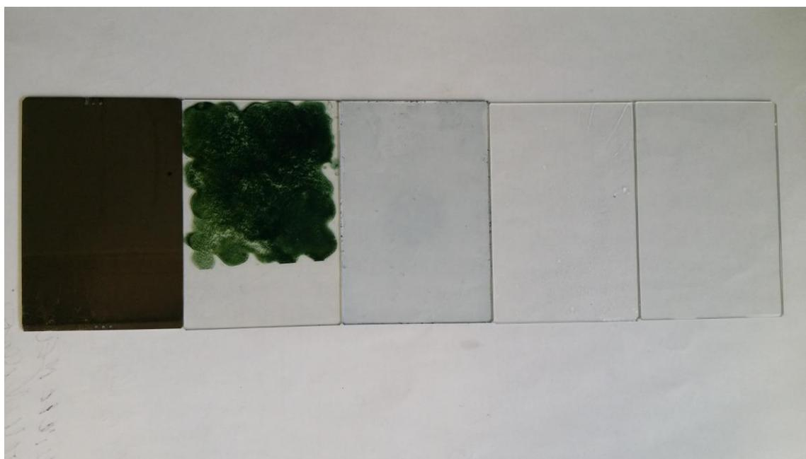
**Figure 13:** From left to right; Pt on Mg<sub>4</sub>Ni, PANI, PEDOT, PEI, and control slide
