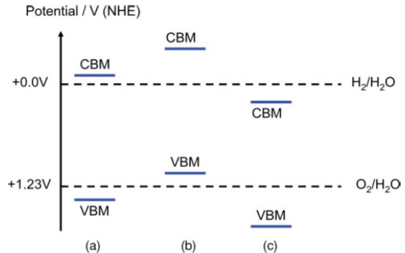
A schematic diagram of possible band level arrangements for water-splitting photocatalysts. a) Favorable band level arrangement b) unfavorable VBM position c) unfavorable CBM position. (Wu 2011).
