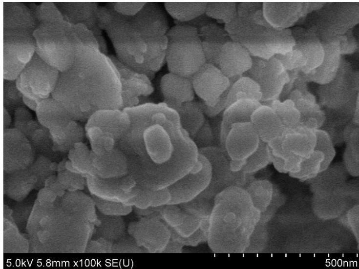
**Figure 16:** This SEM picture shows the relative size and shape of our  $\text{ZnWO}_4$  nanoparticles. The smallest particles, around 20-40 nm, are hypothesized to be our NiO particles.
