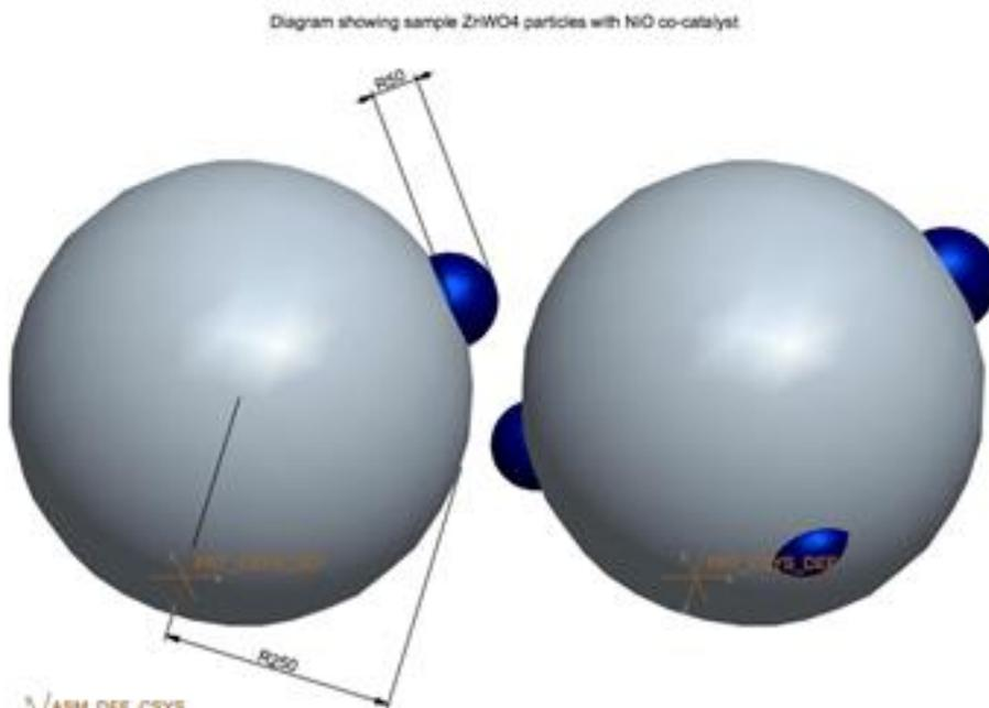
**Figure 3:** Schematic drawing of catalyst structure;  $\text{ZnWO}_4$  (grey) and  $\text{NiO}_x$  (blue); radii are in nanometers (Spherical Shape and  $90^\circ$  contact angle assumed).
