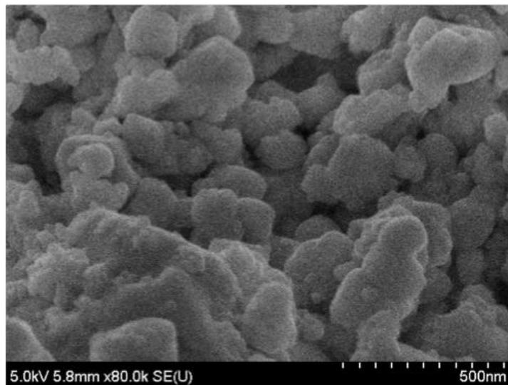
**Figure 11:** SEM output after NiOx deposition.
