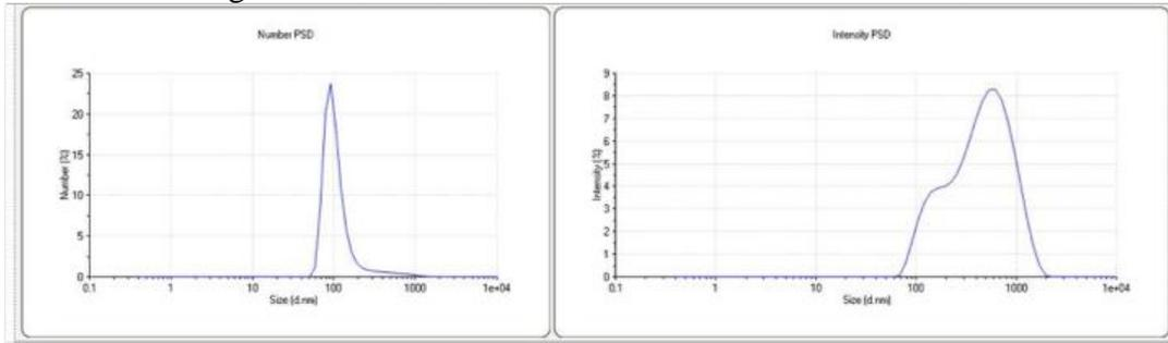
**Figure 10:** Particle Size Distribution (PSD) obtained from Zetasizer Nano; Number PSD (left) and Intensity PSD (right).
