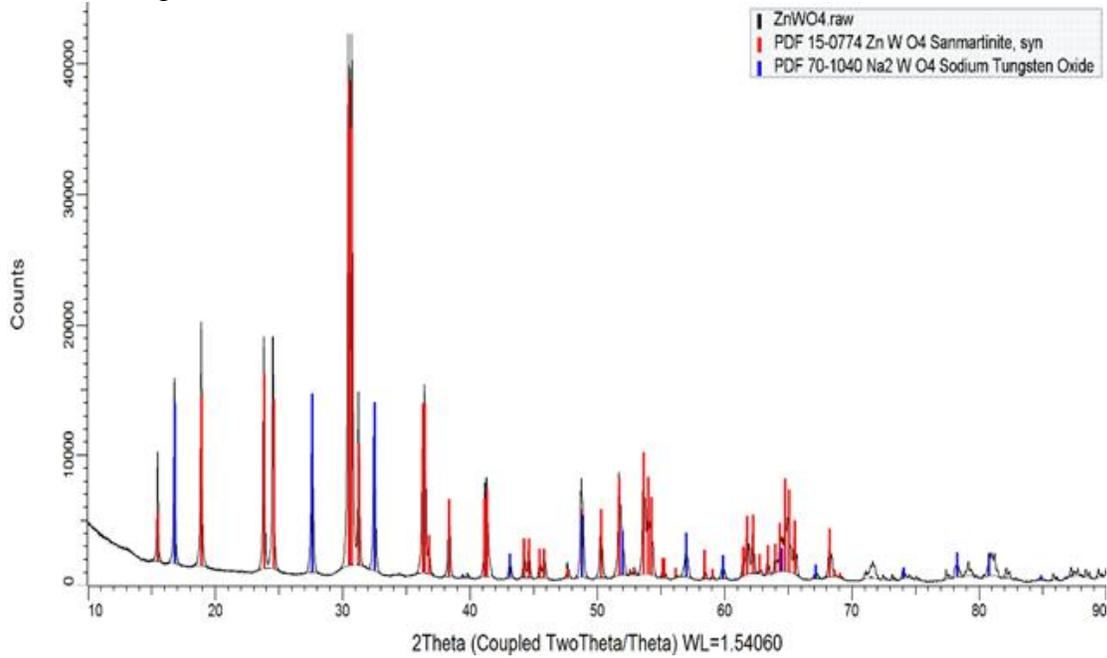
**Figure 9:** Shows the XRD schematic of our first ZnWO<sub>4</sub> sample. The black lines denote the observed spectrum, while the red and blue curves show the ZnWO<sub>4</sub> and Na<sub>2</sub>WO<sub>4</sub> phases respectively.
