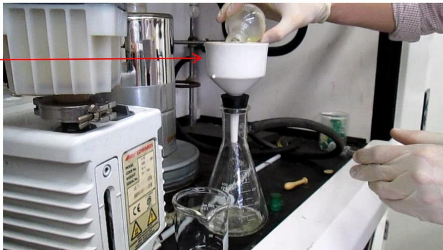
**Figure 16:** Vacuum filtration to remove Sodium Sulfate.
