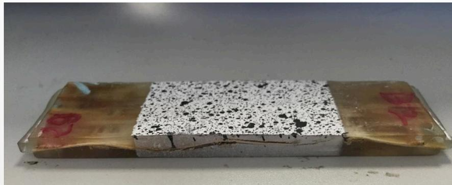
Figure 14: Example of Delamination
