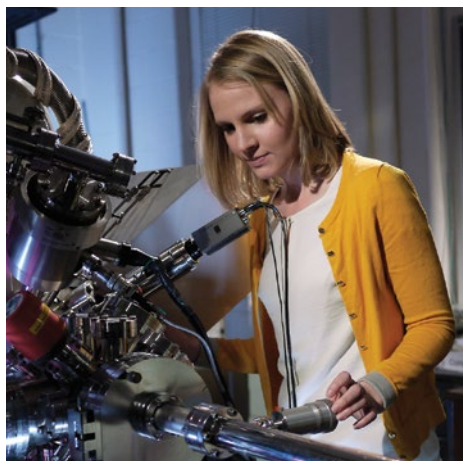
AMY MARQUARDT USING X-RAY PHOTOELECTRON SPECTROSCOPY TO ANALYZE THE SURFACE CHEMISTRY OF SILVER AND BRONZE BEFORE AND AFTER A PROTECTIVE COATING IS APPLIED.
