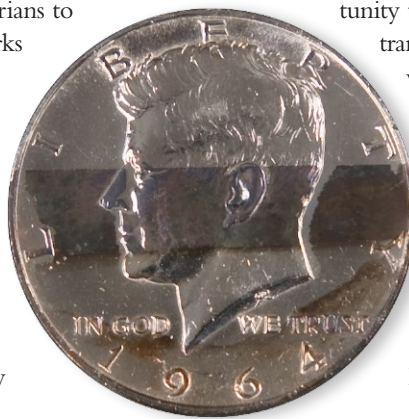
A SILVER HALF-DOLLAR COIN THAT HAS BEEN COATED WITH PLASTIC (BOTTOM 1/3) AND ALD COATING (TOP 1/3). THE CENTER OF THE COIN IS WITHOUT COATING.
