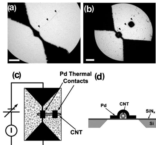
FIG. 1. [(a) and (b)] TEM images of the thermally anchored and unanchored CNT devices used for this study, prior to depositing In with both scale bars of 1  $\mu\text{m}$ . (c) Schematic diagram of thermally anchored device with a circuit overlay. (d) Schematic cross-section of the sample, showing that the CNT touches the  $\text{SiN}_x$  membrane only tangentially whereas the contact of the CNT with the Pd contact width is approximately half the circumference.
